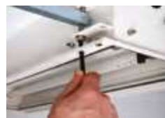
Single screw height adjustment
